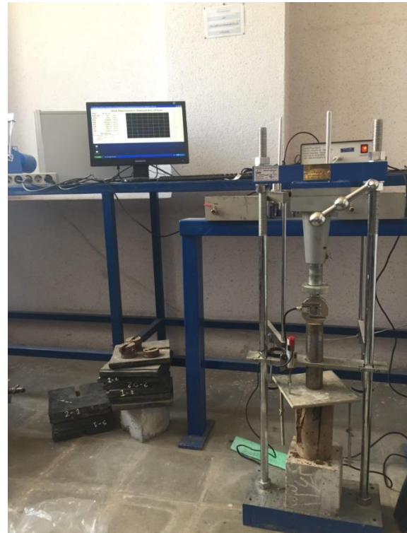
Figure 1. Field sample test under unconfined compressive strength loading and data recording by data logger.
