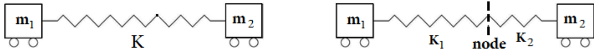
Fig. 1. Dividing the primary spring (left) into two adjusted series springs ( K_1 & K_2 ) from the node location (right)
